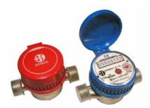
The BONEGA water-meter - S/13 (20) or T/13 (20) is the single-inlet bladed house water-meter for cold and warm water, with internal gate regulation and dry-running counter with a wheel for photometric reading. The water-meter state can be read with precision to 1 litre.
